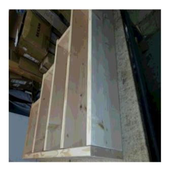
Place The 2" x 12" x 44" Under The 2" x 12" x 9-1/2" Screw Nice And Tight And Screw On To The Size Of The 2" x 12" x 44" As Well. Place the Bottom Shelf On The 2" x 12" x 44" Under The 2" x 12" x 9-1/2" And Screw On To The Side Of The Size Of The 2" x 12" x 44" As Well.
